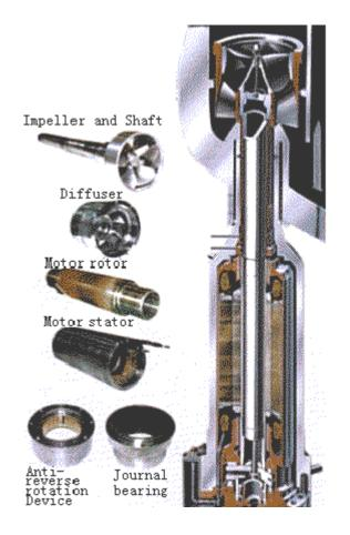
Figure 12. Reactor Internal Pump
