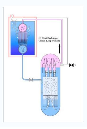
Figure 21. Isolation Condenser System
