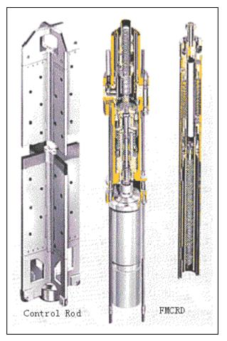
Figure 14. Control Rod and Drive Mechanism
