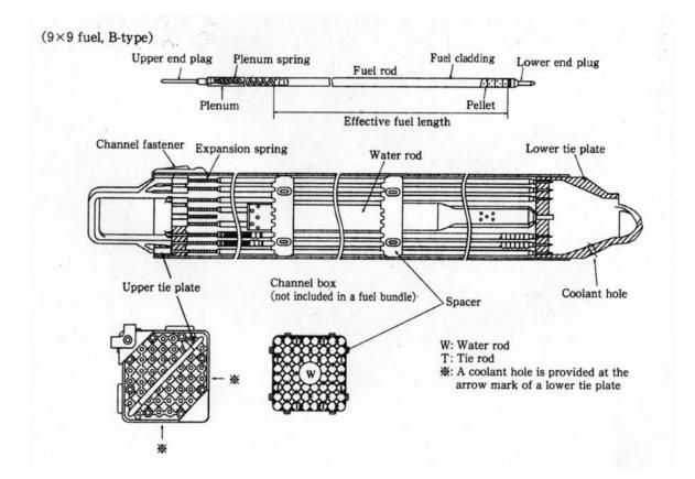
Figure 4. BWR Nuclear Fuel Structure
