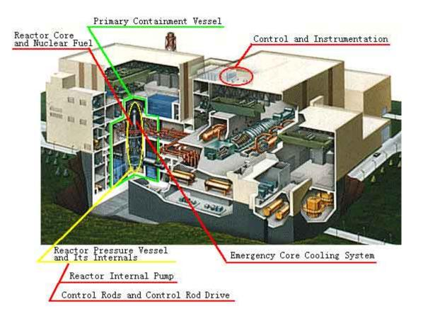
Figure 8. ABWR Power Plant Structure
