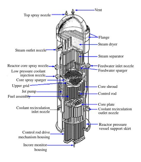
Figure 3. Internal Structure of BWR Reactor Vessel
