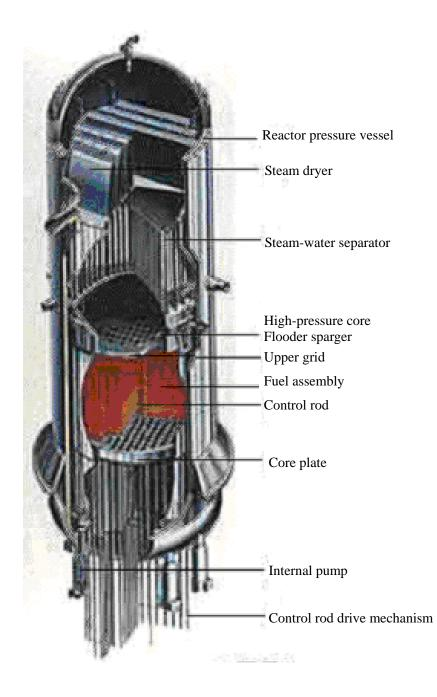
**Figure 9. Reactor Pressure Vessel and Internals**
