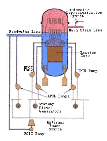
Figure 15. Emergency Core Cooling System (ECCS)
