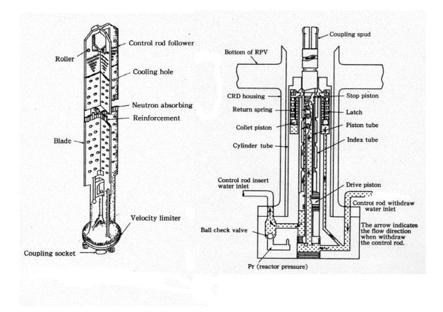
Figure 5. BWR Control Rod and its Drive Mechanism
