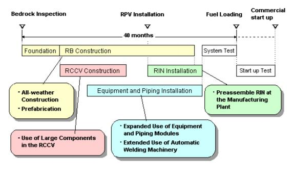
RCCV: Reinforced Concrete Containment Vessel RPV: Reactor Pressure Vessel RIN: Reactor Internals RB: Reactor Building
