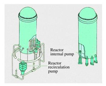
Figure 11. Reactor Cooling Pump for BWR and ABWR
